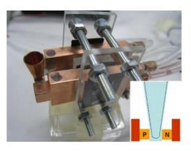
Fig.1 Photograph of our Peltier device and (inset) schematic structure of our PN-sandwiched well block.
