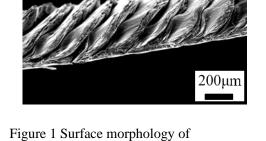
Zr<sub>55</sub>Al<sub>10</sub>Ni<sub>5</sub>Cu<sub>30</sub> metallic glass wool (fiber).
