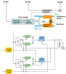
Fig. 2 Schematic structure of our PCR system
