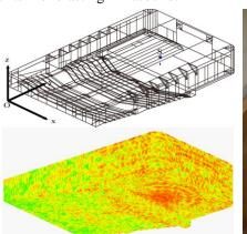
Figure 2. SPL distribution obtained by the fast multipole boundary element method.
