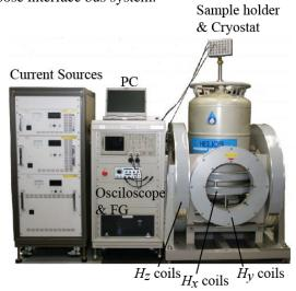
Figure 1 Measuring System
