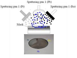
Fig. 2 Sputtered plates with threeguns sputtering equipment to prepare high throughput screening of electrocatalysts for fuel
