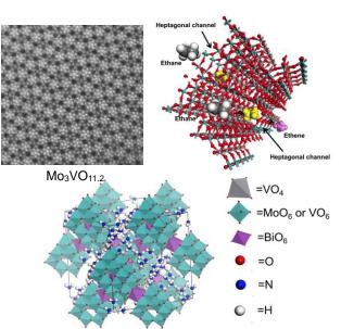
Figure 1. Examples of high-dimensionally structured metal oxide catalysts
