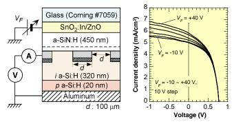
Field-effect solar cell and its J-V characteristics
