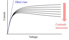
Figure 2. I-V curve of the average electric current in the interacting resonant-level model.
