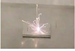
Figure 2 MOPA fiber laser machining.
