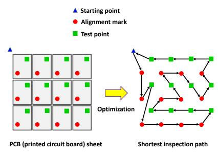
Figure 1. Path optimization for PCB inspection
