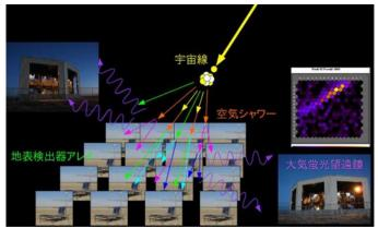
Fig 1: Schematic view of the extended air shower and detectors of SD array and FD telescope.
